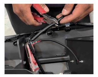
18. Then connect the Black wires together and the Yellow and Red wires together to connect the Number Plate Light. Solder and wrap in electrical tape to finish.
