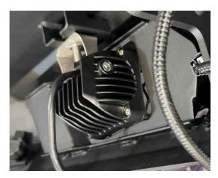
14. Plug in the Sensor Plugs from the Factory Harness to the Sensors that were fitted on the Rear Bar. Depending on how many sensors the vehicle has, different sensor plugs will need extending.
