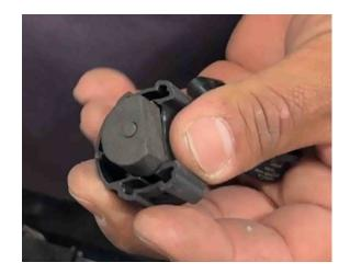
10. Put the Sensor into the Sensor Chambers that were fitted on the Rear Bar, making sure the positions of the sensors that were on the factory bar corresponds with the positions on the Supreme Rear Bar. Then place the Chamber Lid on top to secure it.
