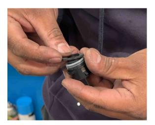
9. Take the Semi-Circle Foam Sticker and attach that to the Sensor Chamber Lid as shown.
