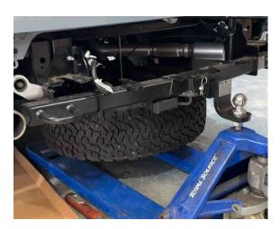
21. Unscrew the Exhaust attachment to make the next steps easier. Don't need to remove, just unscrewed so the Exhaust is flexible and can be moved out of the way. Do this for both sides.
