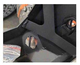
6. Fit the Sensor Chambers to the Sensor Holes on the Rear Bar, Chamber on the inside, Ring Cover on the outside.
