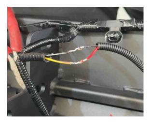
19. Cable tie the Factory Harness to the Rear Bar so the Sensors do not move even if the Harness moves.
