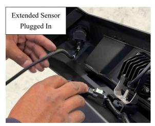
16. For vehicles with 6 Sensors, use the factory harness plugs to connect the 2 furthest outer sensors, the 2 inner most sensors, then extend the 2 sensors that are between outer and inner most sensors with the Extension Cables. Neatly fold and cable tie the extension cables to the bar.
