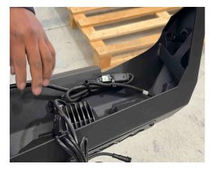
17. Shorten the Number Plate Light cable on the Supreme Rear Bar exposing the Red and Black Wires. Then cut and expose the Factory Harness Number Plate Light Wires which are Black and Yellow.
