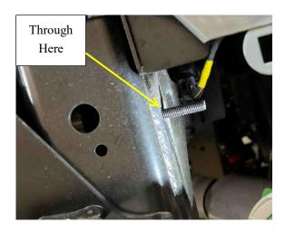
29. Then secure the smaller L Shaped bolt with a Flat Washer, Spring Washer and Nut.
