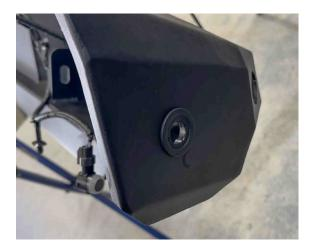
7. Detach Sensor from the Harness and remove the white ring cover on it.
