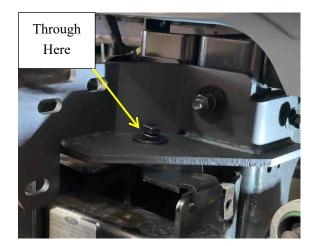
32. Measure the distance between the brackets on the rear bar, then measure the distance between the Brackets that were setup above. Adjust the Bracket setup so the distance allows for the Rear Bar brackets to fit.
