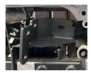
28. Use the smaller L Shaped Bolt to go through the hole shown, reach in through the back and from the bottom up (Bracket from step (27) not shown here, but it needs to be on with the spacers with this bolt going through).
