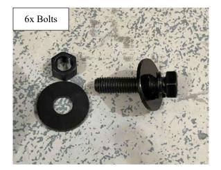
35. Secure the Rear Bar to the Brackets with the 6 bolts shown above, 3 bolts per side.
