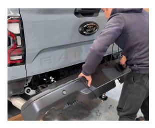
3. Cut off these pieces shown below on both sides of the vehicle. Spray the cut edge with an anti-rust paint to prevent rusting.
