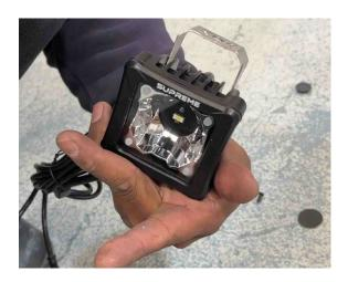
13. Setup the Cube Light Bracket like shown (If you can use a bigger washer like the black one shown – this is not provided) and fit the Bube Light onto the Rear Bar making sure to aim the Cube Lights downwards.
