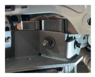
31. Setup a Bolt like this, then it goes through the bottom hole bracket and spacer and secure with flat washer and nut. DO NOT tighten anything completely yet, adjusting still needs to be done. Setup both Brackets.
