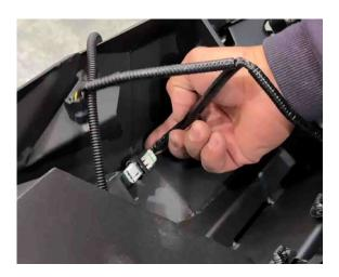
15. For vehicles with 4 Sensors. Plug in one side sensor and the 2 middle sensors with the factory harness sensor plugs. Extend the furthest side sensor plug with the extension cable provided.
