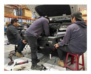
41. Use Bolt (E) Setup from Step (10) to secure the Front Bar to the Cradle Bracket (Do NOT Tighten yet, this will hold the bar in place for adjustments). Adjust the Front Bar as even as possible and leave a 15-20mm gap between the Bar and the Vehicle's Head Lights. Leave a 25-30mm gap between the Bar and the flares on the sides. This will prevent flexing damage to the vehicle. Tighten Bolts when positioned.
