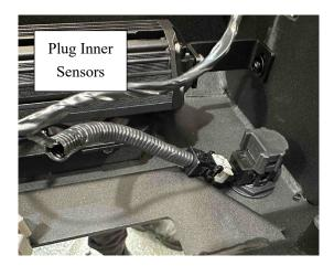
36. The Outer Sensors will be out of reach, you will need to extend the Sensor harness Wires. Start by splicing and exposing the Red Green and Blue Wires. Cut them and extend the wires long enough to reach the outer sensors and plug the Outer Sensors in.
