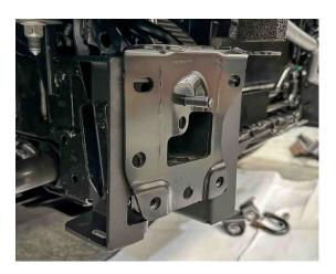
12. Sit the Winch Cradle in place on top of the Recoveries and secure with Bolt (C) on both sides (But don't tighten yet).
