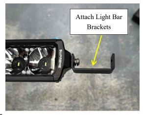
26. Get the Light Bar into position and adjust the angle so that it is aiming slightly upwards. Then tighten the Bracket with the bolts.
