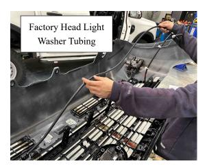
35. Remove all the hard plastics and wrappings around the Factory Light & Sensor Harness and relocate the Harness to the Supreme Bar and plug in the inner Sensors
