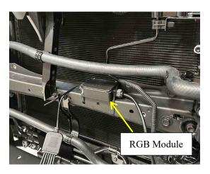
19. Unplug the Factory Head Light Socket on the Driver's Side. Located the Purple/Light Purple Wire (Signal Light Wire) and extended it about 80cm. Do the same for the Passenger's side but the wire will be Purple/Blue coloured.
