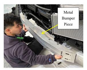
9. Remove the Factory Recovery Point. IMPORTANT: Keep the 4 Factory Bolts from the Recovery.
