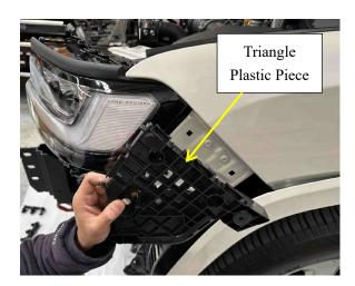
5. Remove the plastic side grille pieces and plastic covers around the intercoolers on both sides.
