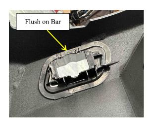
31. Remove the Front Cover on the Head Light Washer and discard Cover. Fit the Head Light Washer onto the Supreme Bar attached to the casing, then Cover the front of the Head Light Washer with the Supreme Washer Cover provided.
