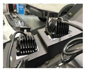
**NOTE:** When tightening the cube lights into position, make sure the light is NOT touching the frame of the bar, and that it is facing forwards as straight as possible and aiming at a slightly down angle.
