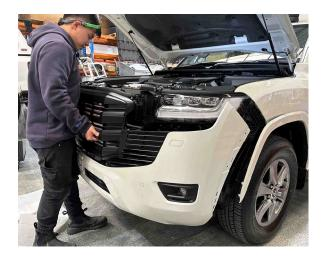
4. Remove the triangle plastic piece that's next to the head light and flares as shown for both sides.
