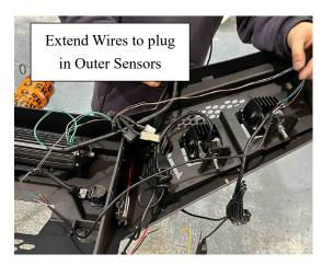
37. Connecting the Cube Lights to the Factory Harness: Connect the Black Wires from both Cube Lights to the White Wire of the Factory Harness, then the Red Wire from both Cube Lights to the Green Wire of the Factory Harness. The Blue Wire from the Outer Cube Light does NOTHING, so just cut it and neatly bind somewhere (Can tape it to the yellow like shown below NOT connected, just taped).
